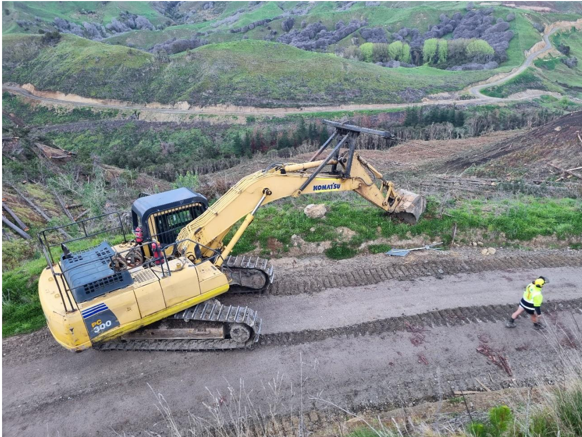
Photo 1: T-bar tail hold repositioned and ready for next haul section.
