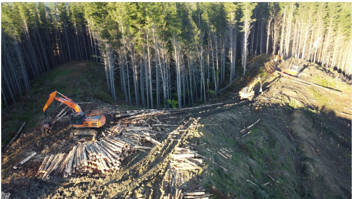
Photo 6: The two-stage set up where logs are moved from the swing yarder to the processor.
