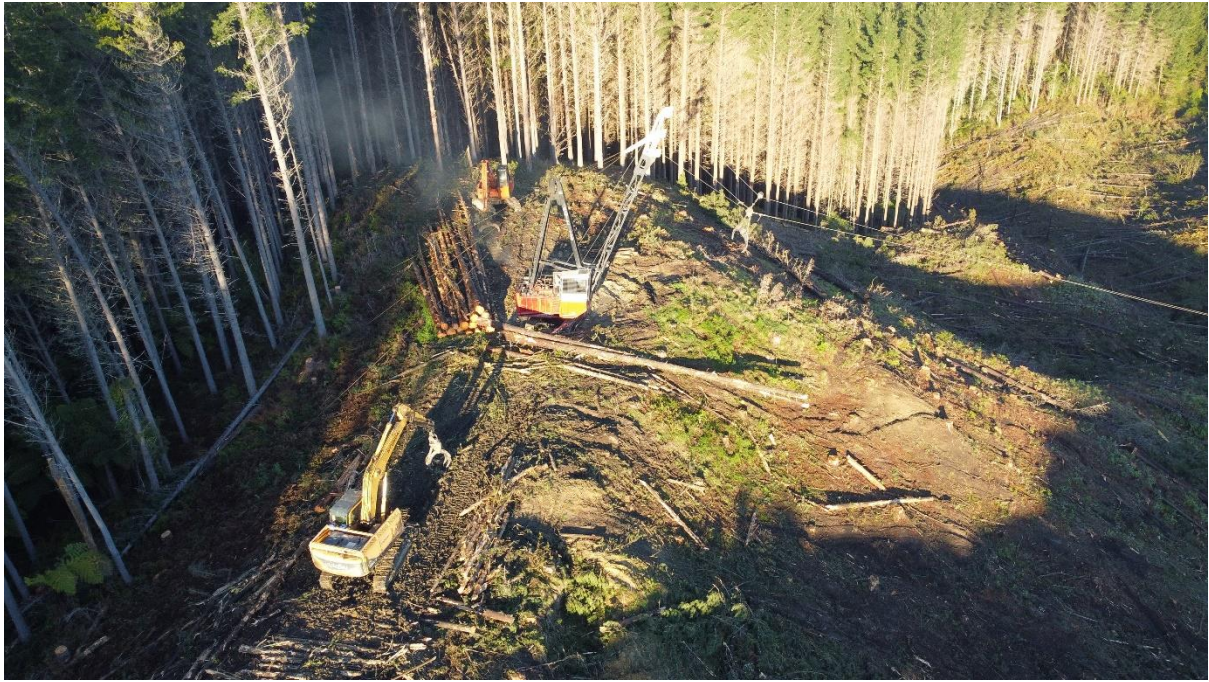
Photo 7: Aerial view of the swing yarder on Pad 28.
