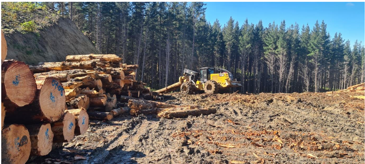
Photo 2: Skidder pulling stems to Landing 11.
