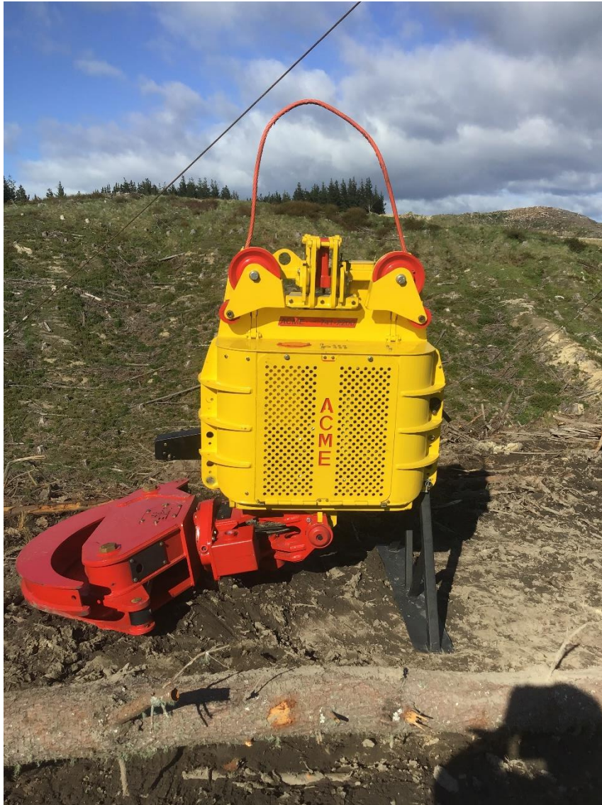
Photo 6: New Acme claw to be run on hauler to minimise men on the ground to help with safety.
