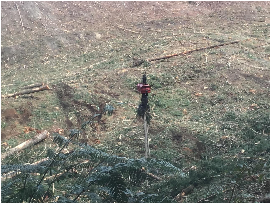
Photos 1 & 2: Grapple with motorised carriage pulling a drag back to the harvestline in Setting 92.
