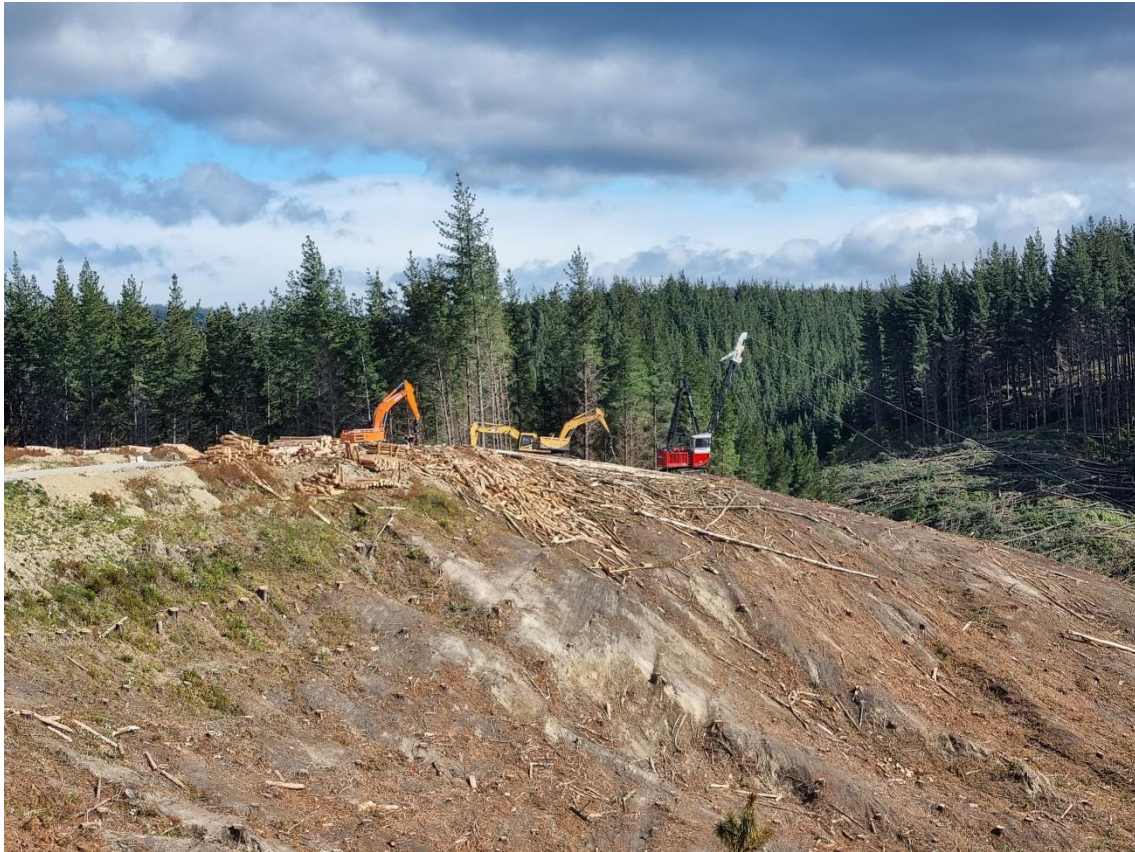
Photo 1: Machines walking stems from the swing yarder up to the processor.
