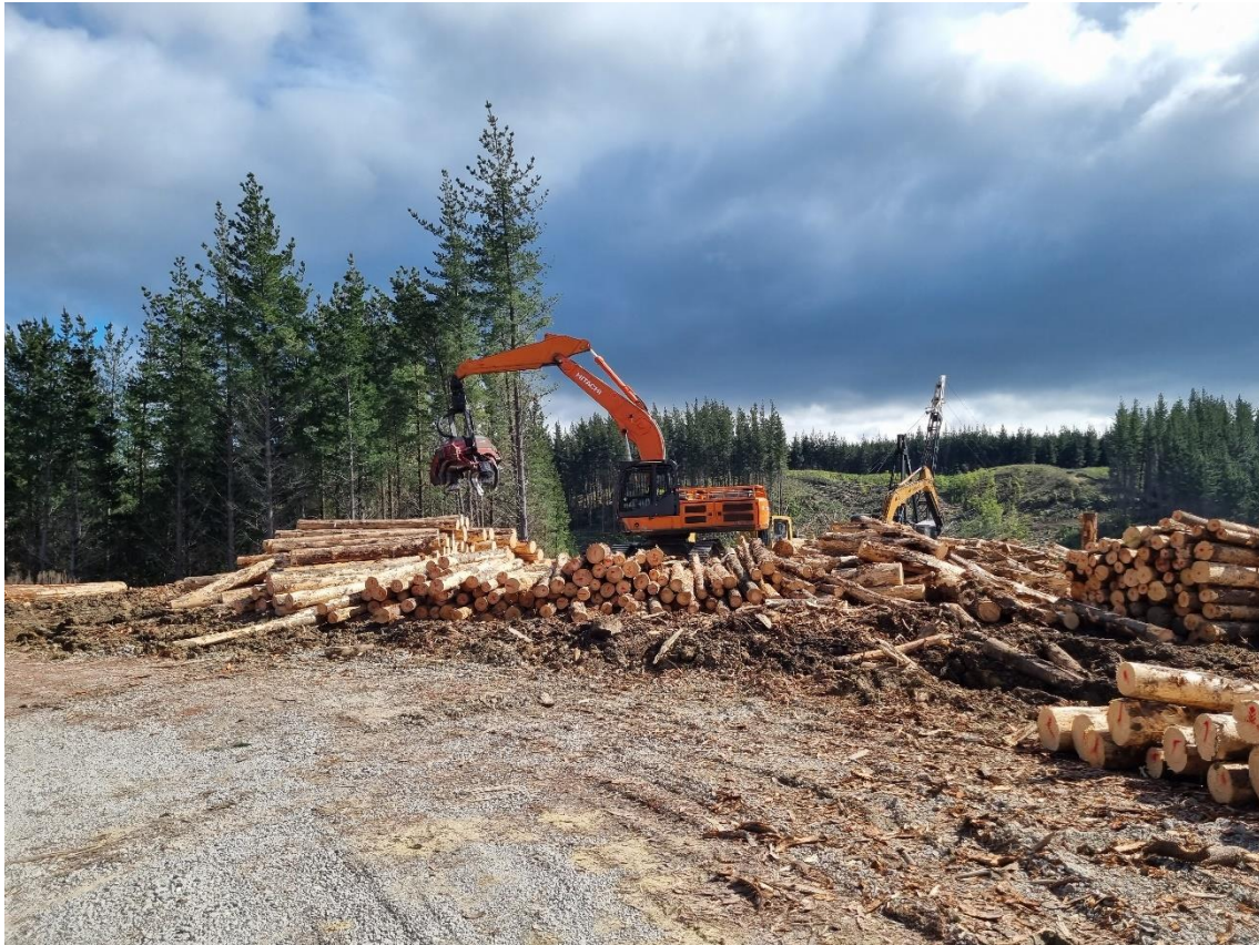
Photo 3: Processor cutting logs and dropping into piles to be stacked.
