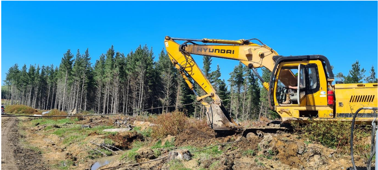
Photo 1: Anchor machine in position for the swing yarder in Landing 30.
