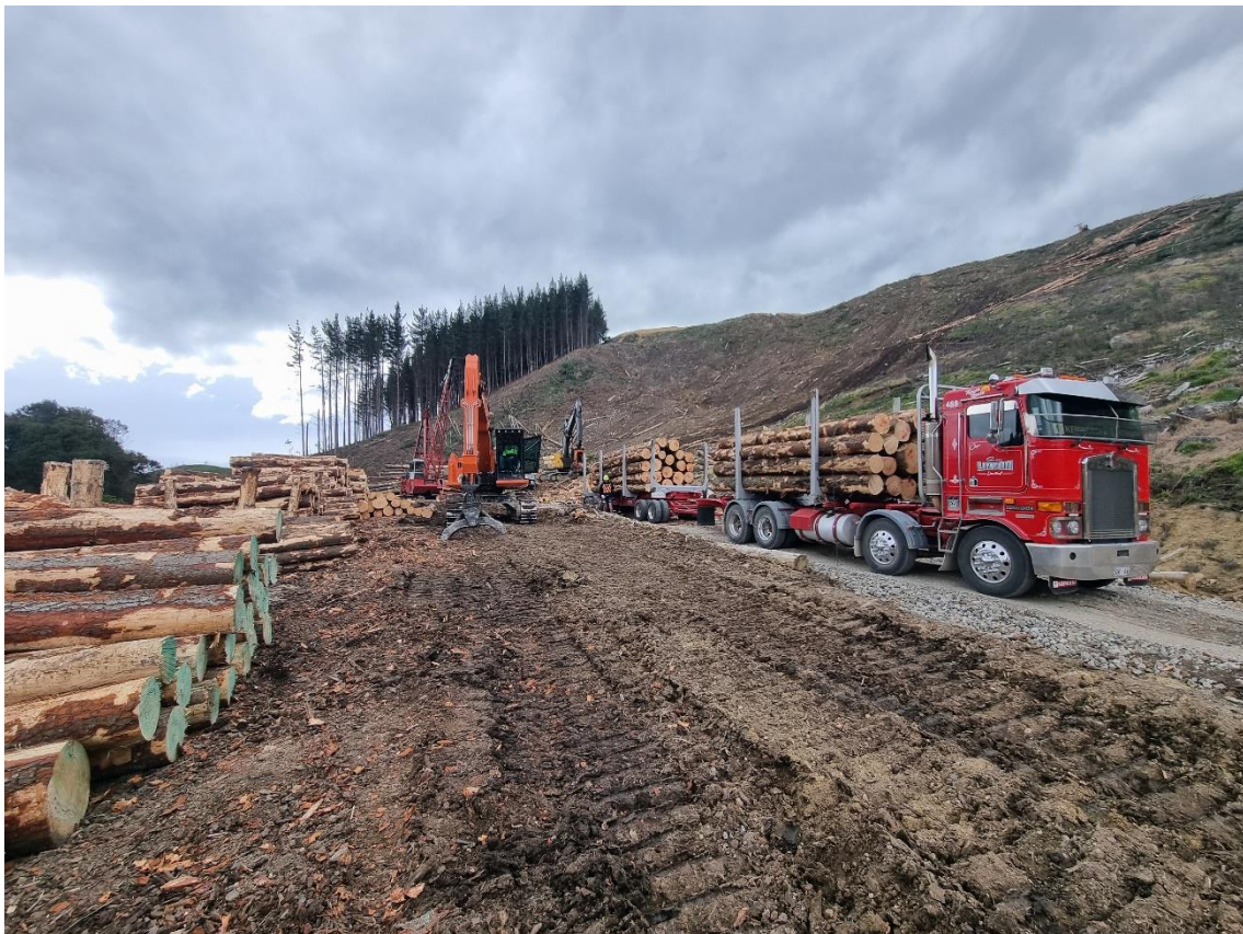
Photo 6: Loaded truck carrying out a stack check before leaving the landing. Loader driver stationary, staying safe.
