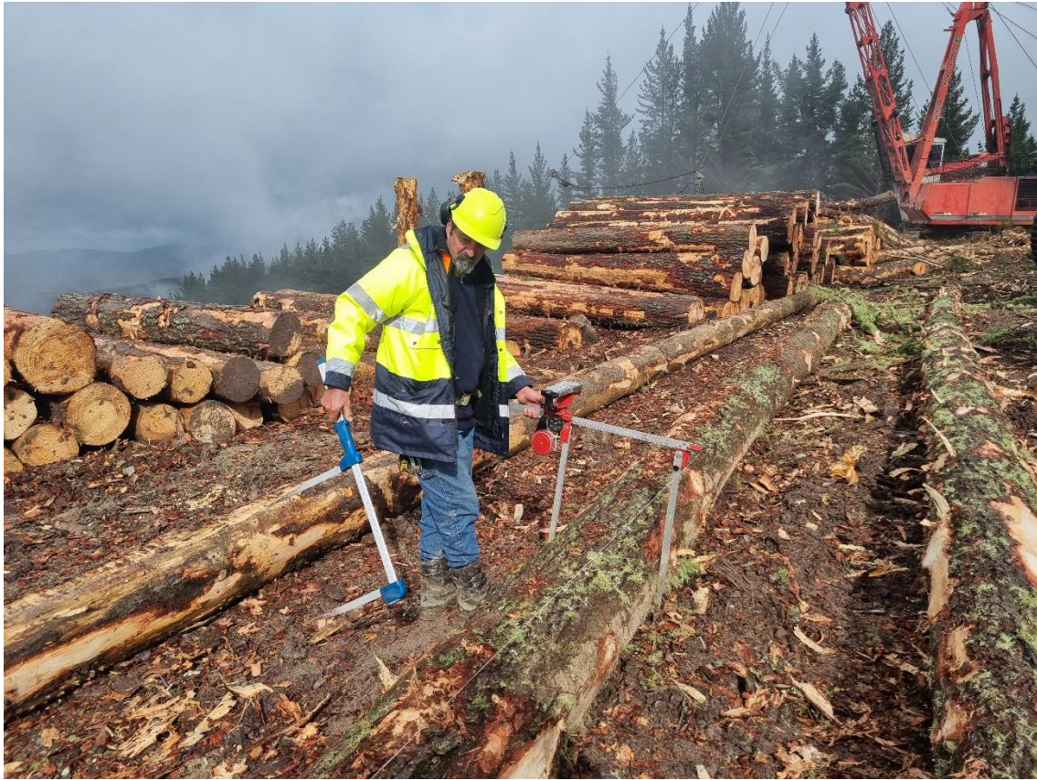
Photo 3: Log Value Recovery audit being carried out on processor operator.
