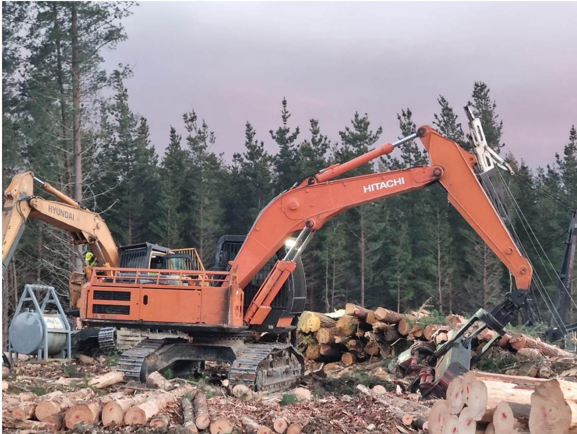
Photo 3: Shovel machine being fuelled up and processor being maintained on Landing 28.
