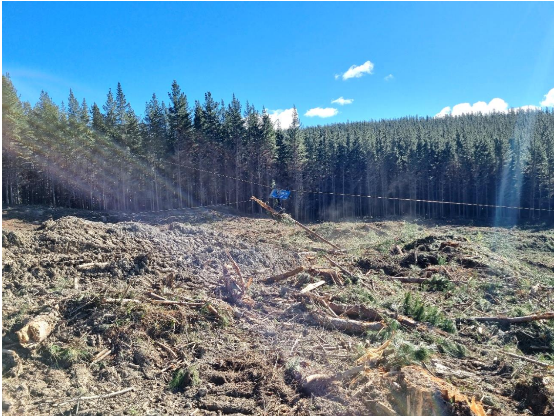
Photo 1: Log 11 grapple carriage flying through the air to retrieve next drag.
