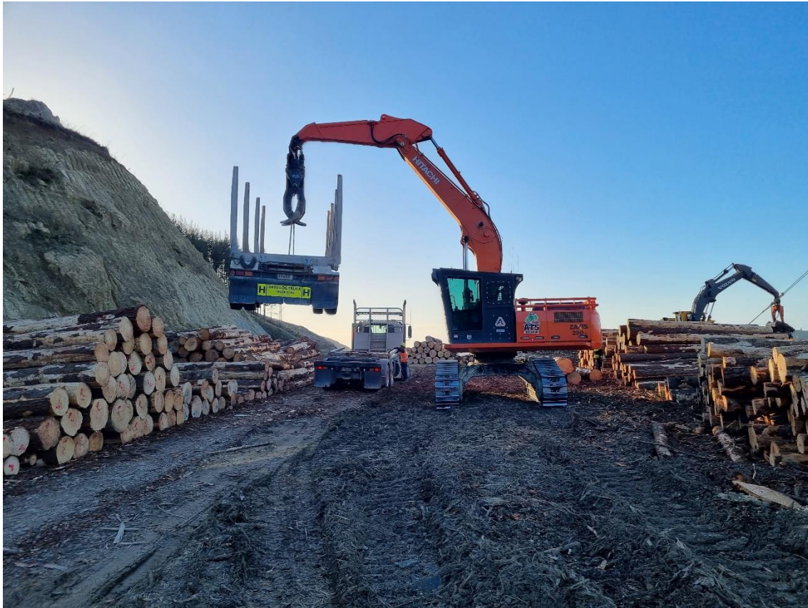
Photo 3: Loader lifting trailer off truck for loading.
