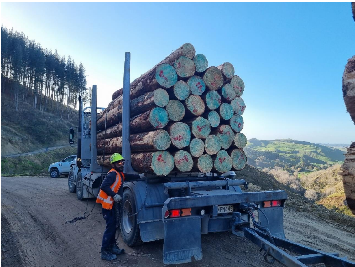
Photo 4: Driver chaining up loaded truck.
