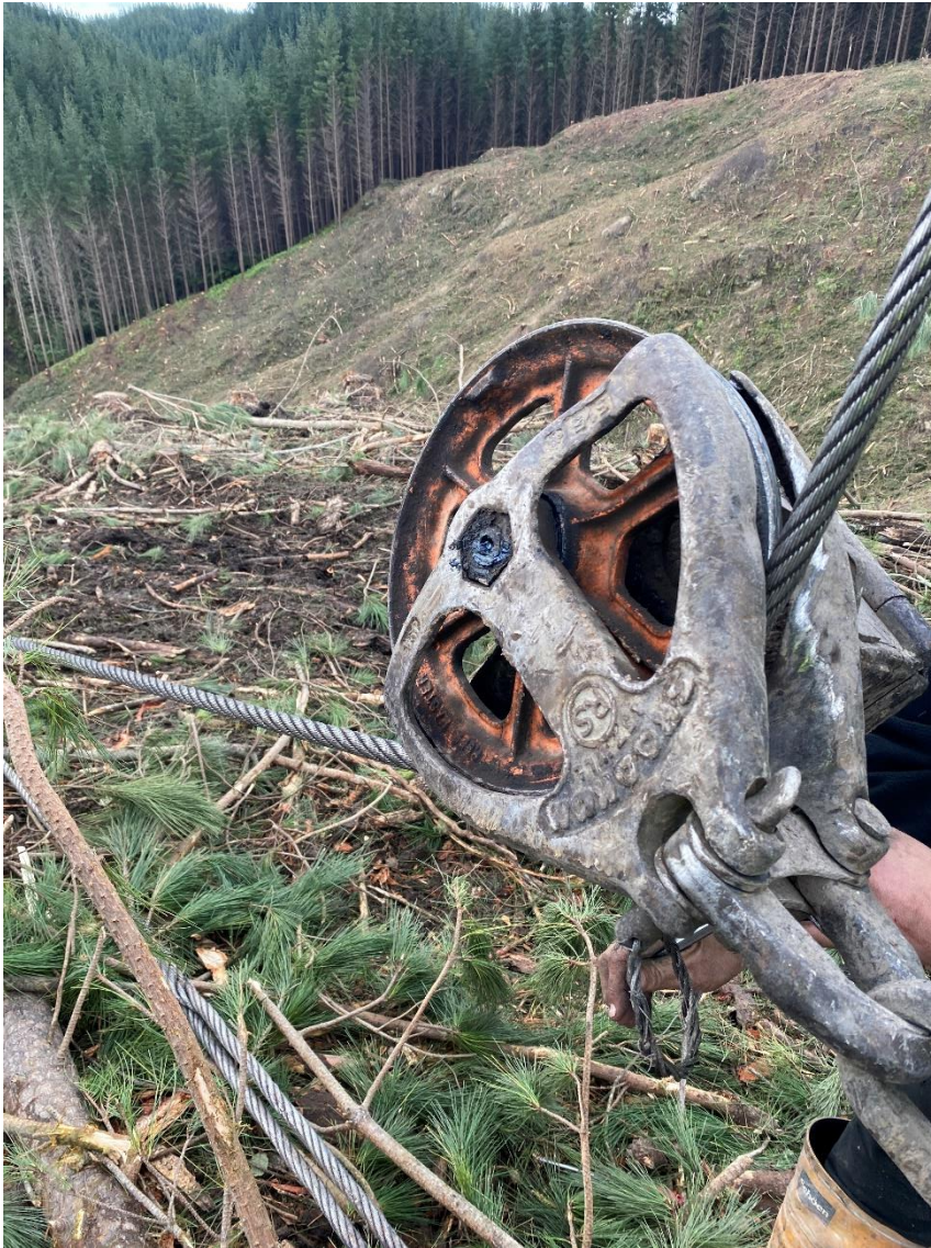
Photo 7: Block on the grapple which the wire rope gets pulled through.
