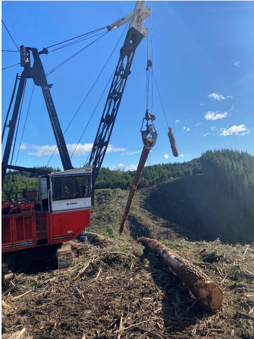
Photo 8: Drag being pulled in by the Log 12 swing yarder in Setting 30.
