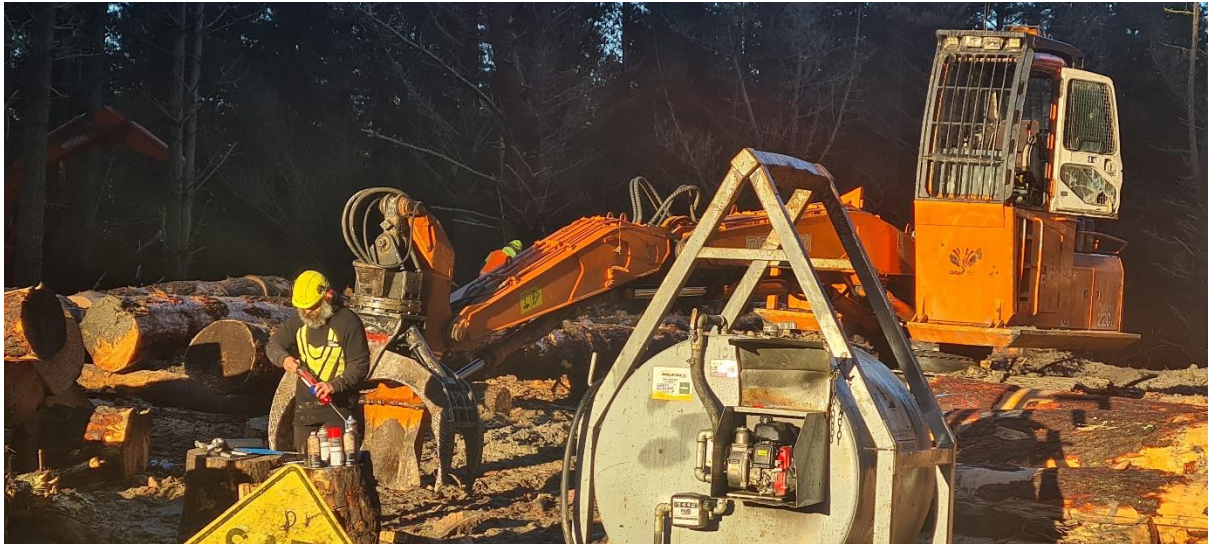
Photo 4: Log 13 crew member about to grease their grapple, on Siobhan Road.
