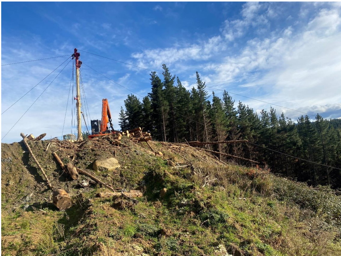
Photo 2: Processor sitting under the hauler in Setting 18 processing stems into logs.
