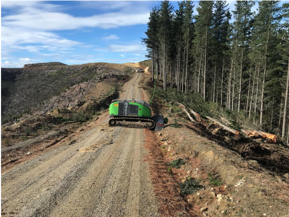
Photo 1: Tethered base machine on Cedar Road.
