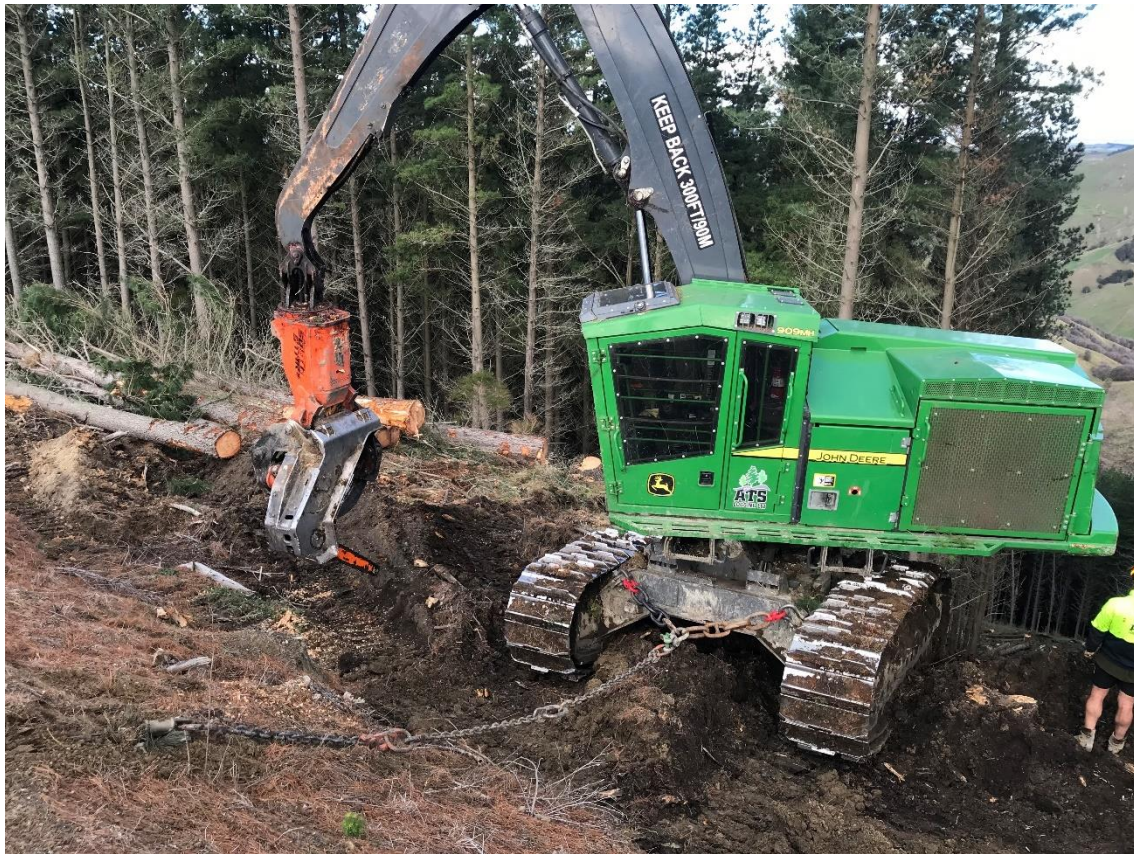
Photo 3: Harvester set up for tethering.
