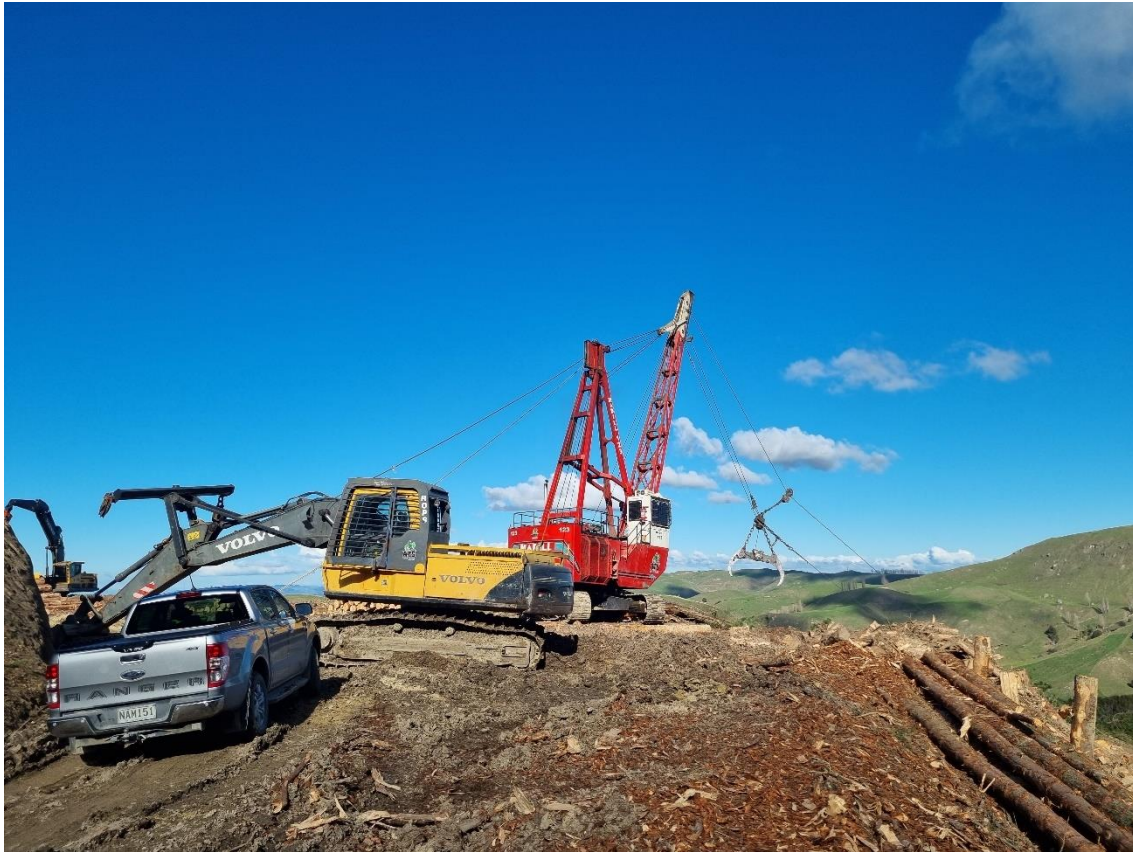
Photo 5: Swing yarder with machine used as an anchor.
