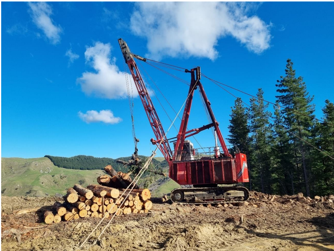
Photo 8: Swing yarder bringing loads up to be placed on landing.
