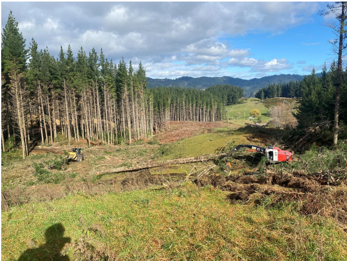
Photo 3: Felling machine feeding stems to the skidder in Setting 4.
