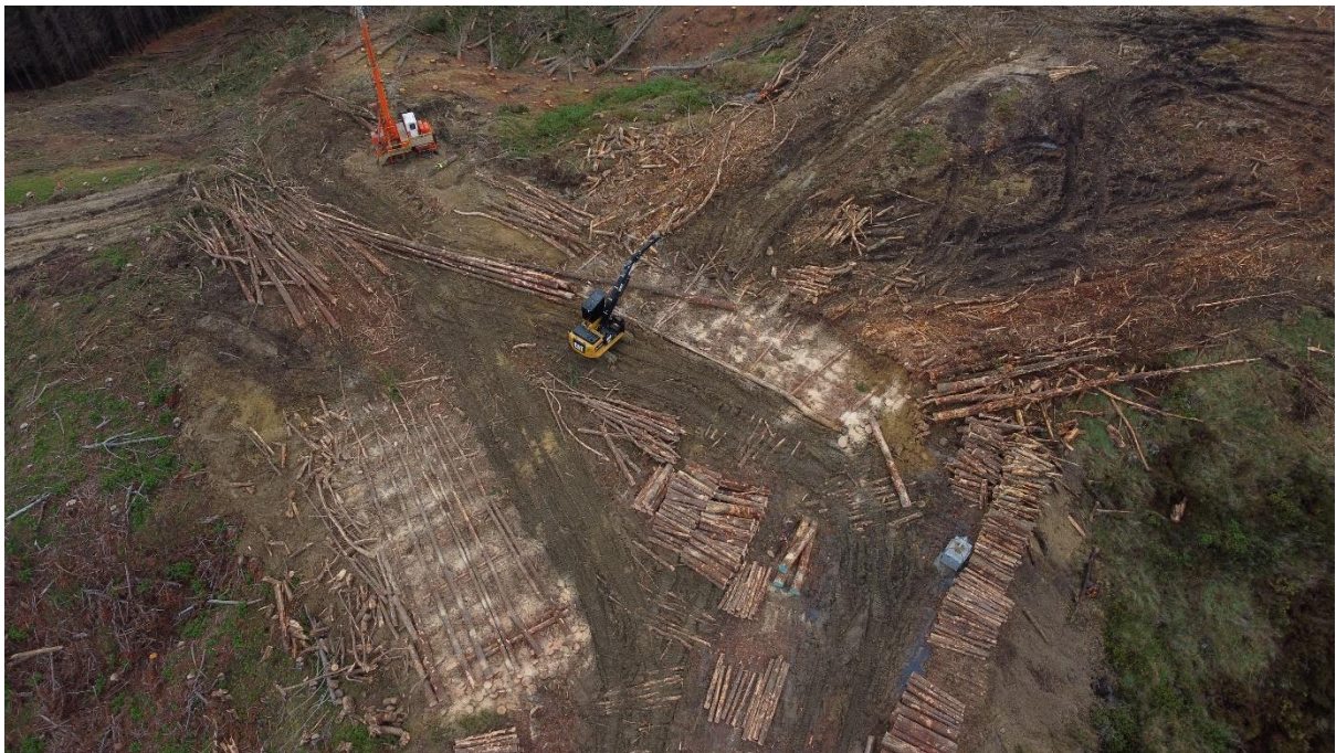
Photo 6: Loader laying out a deck of stems for manual processing on Landing 3.
