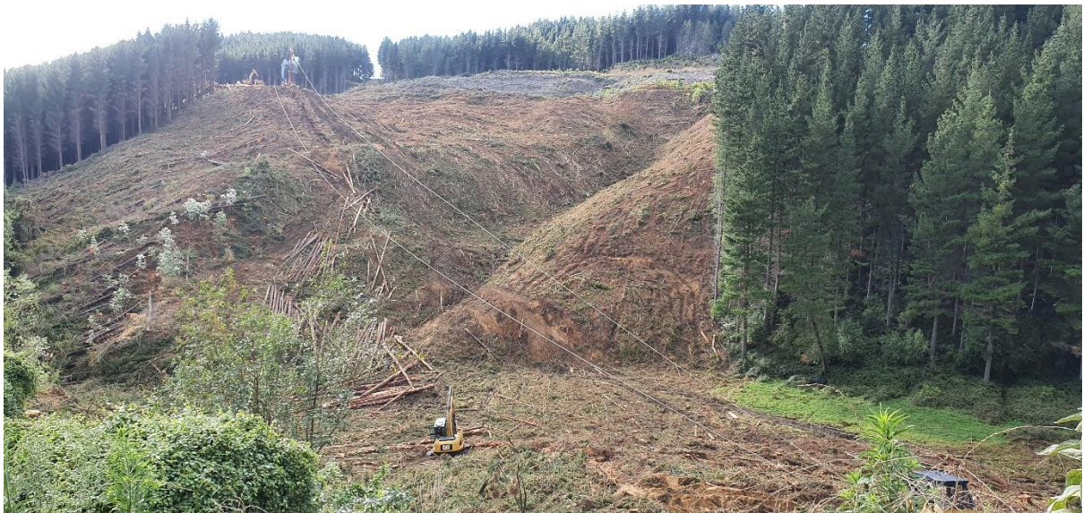
Photos 3 & 4: Hauler skyline stretched out over Setting 82 for grapple to haul stems back to landing.
