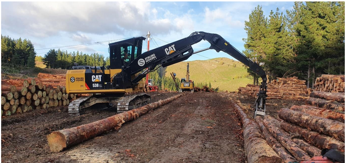
Photo 2: Hauler pulling in a drag of two stems behind the loader on Landing 82.
