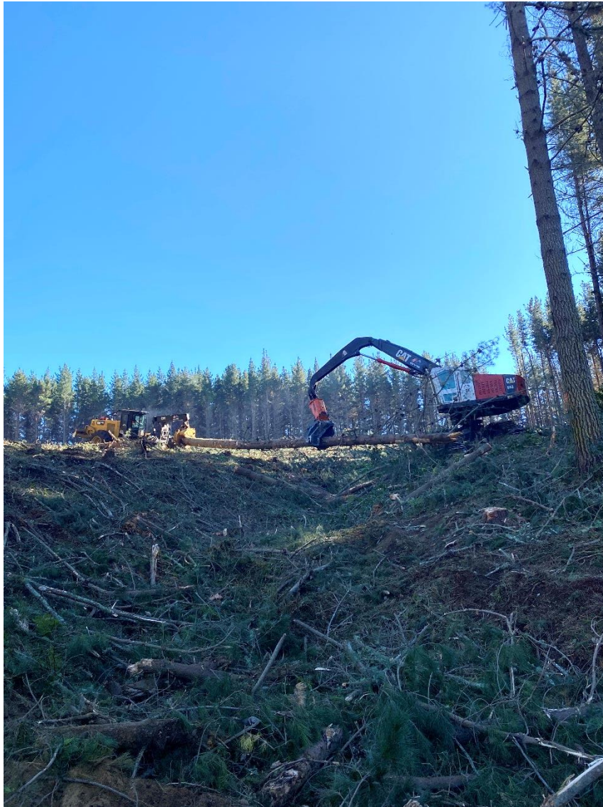
Photo 1: Log 17 felling machine shovelling trees to the skidder to be pulled to Landing T1 for processing.
