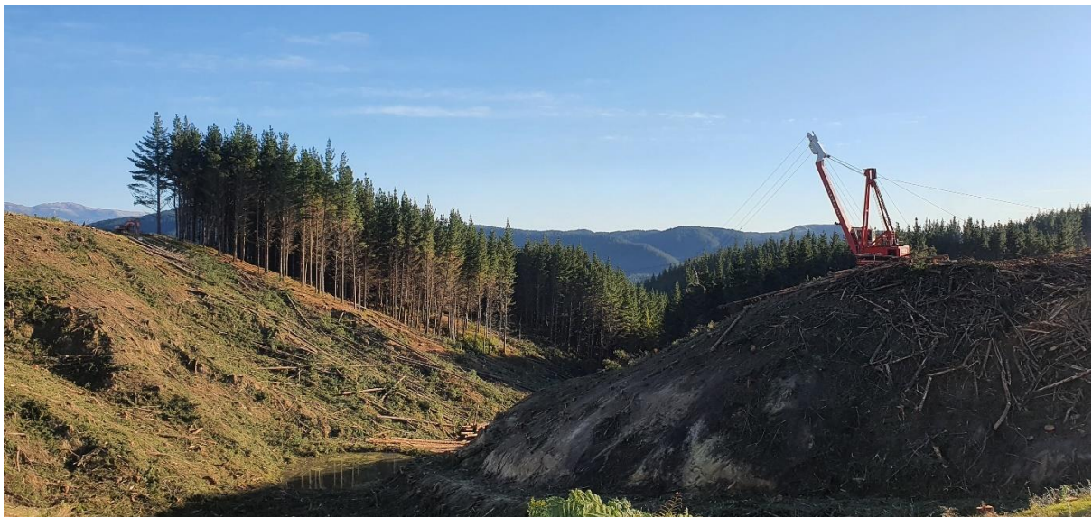
Photo 4: Log 1 extracting stems with swing yarder to Pad 1A.
